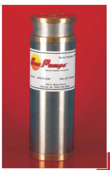
**SunPumps** SDS series submersible pumps are highly efficient, low voltage, DC powered, diaphragm type positive displacement pumps designed specifically for water delivery in remote locations.
