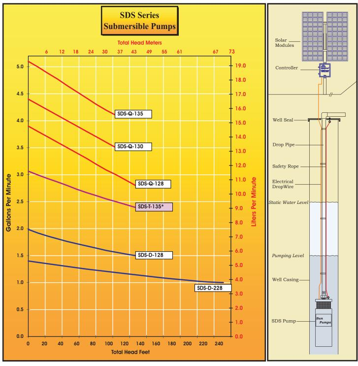
\* SDS-T series pumps are supplied with Super-Tuff Delrin end bells instead of bronze.
